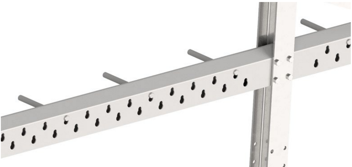
SP-CER consists of one or two rows of crossbeams which are provided with “keyholes” these keyholes are designed so that the steel mandrel can be easily placed where this is desired, while the mandrel is locked, we recommend that plastic or wooden wedges are used between the mandrel and element.
