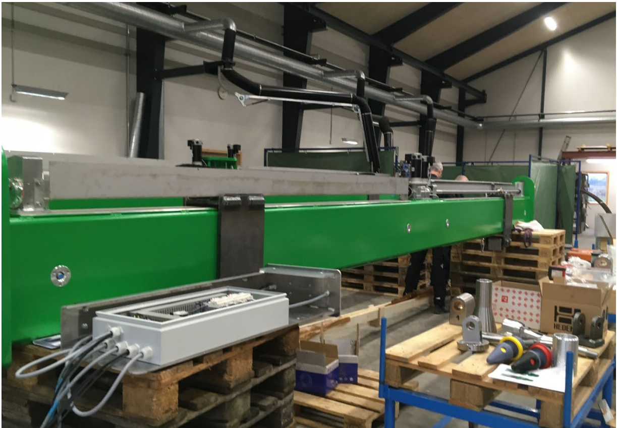
Lifting yokes are assembled and tested.
