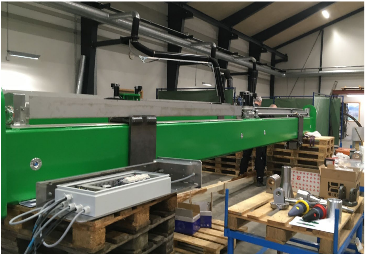
Lifting yokes are assembled and tested.
