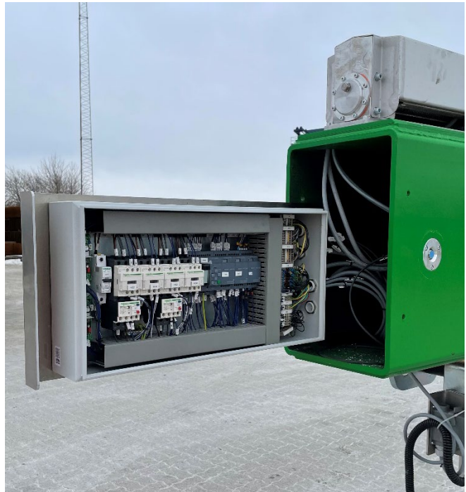
Control board is placed in the yoke on slide rails
